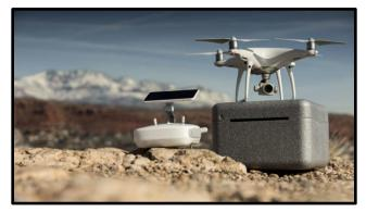
capture large amounts of data in relatively short periods of time. Drone surveys are ideal for providing incremental surveys to monitor construction progress or provide volumetric calculations for stockpiles or other masses.
