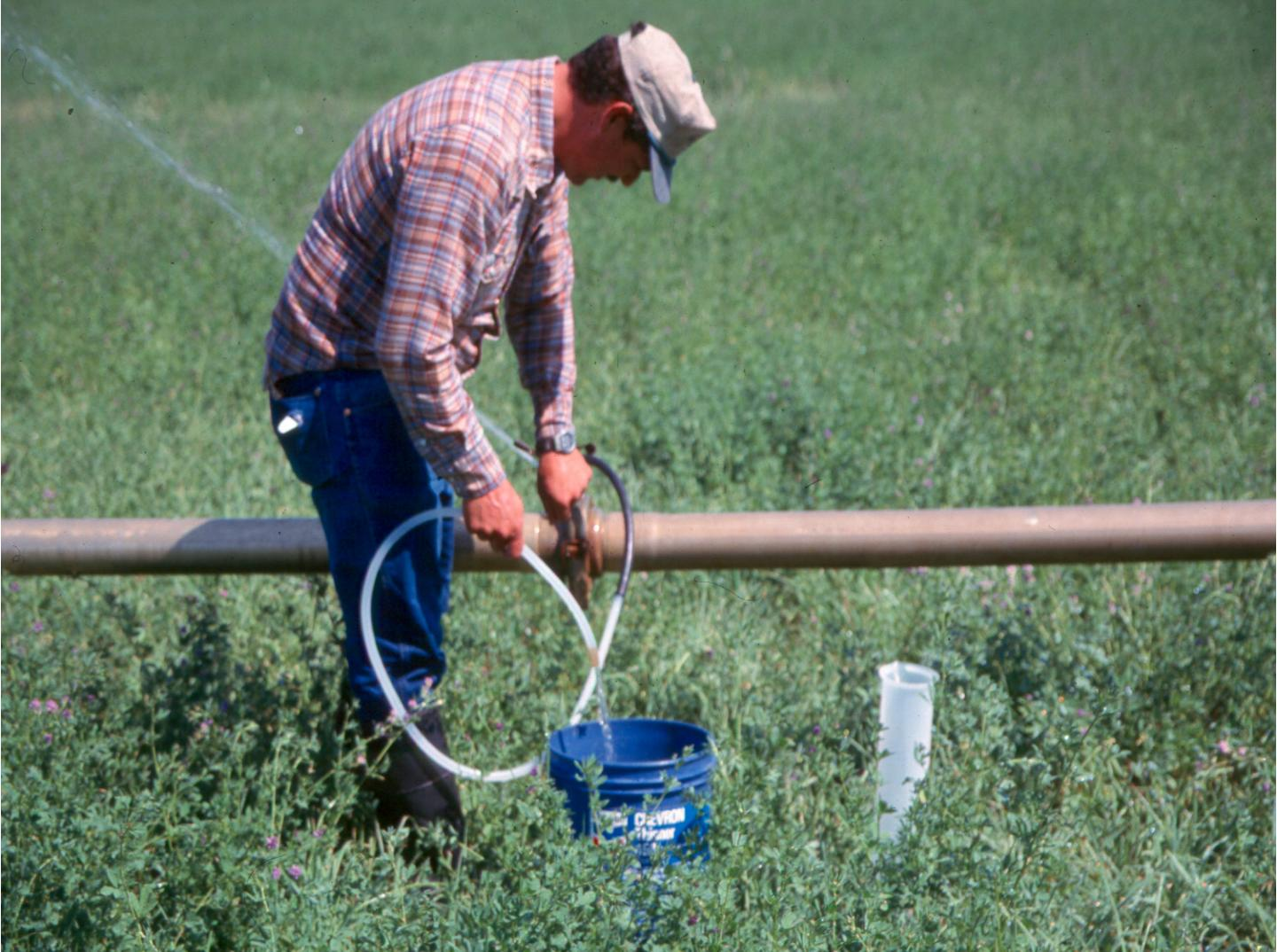
**Flow per nozzle and nozzle size and pressure**
